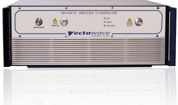
The amplifier operates in class A, the benefits for EMC applications being very low distortion and tolerance of 100% mismatch. Fold-back protection is neither fitted nor needed! This makes it supremely suited for very demanding transducer and test chamber requirements.
